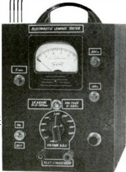
This checker tests electrolytics.
