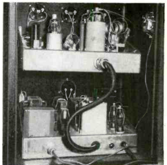
The two 813's and the plate coil are shown in the photo at the left. On the right the r.f. chassis is on the top, with the power supply-modulator below.
